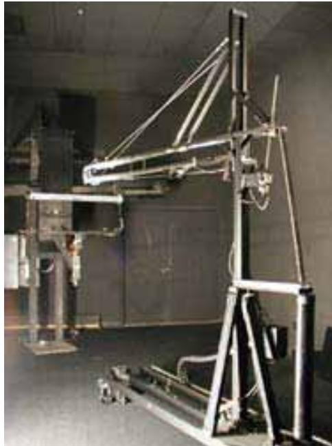
Figure 3 shows the section view of geometry coordinate system of the linear moving-detector photometer where the traveling range of photo-detector/robot-boom is illustrated. During the photometric measurement process, the maximum travel distance between the photo-detector and luminaire is set to be 3.05m (10ft) for both horizontal-axis (Y) and vertical-axis (Z).
